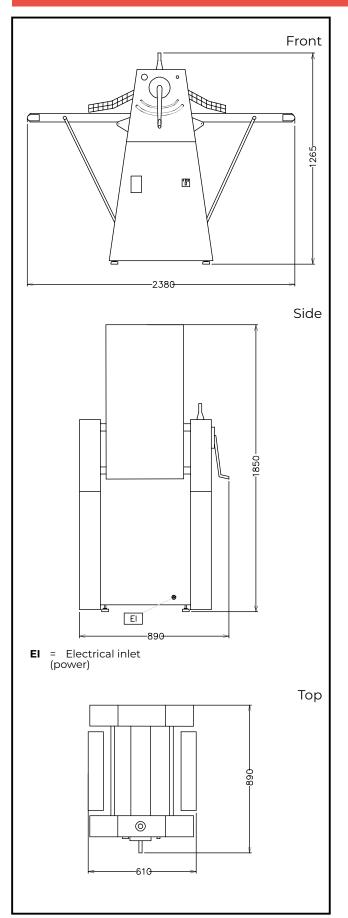
Electric Supply voltage: 230/400 V/3 ph/50/60 Hz **Total Watts:** 0.75 kW Key Information: External dimensions, Width: 2380 mm External dimensions, Depth: 890 mm External dimensions, 1265 mm Height: Net weight (kg): 160
